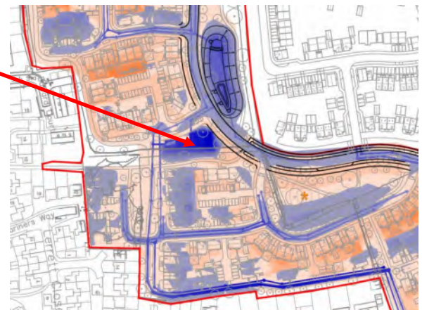
Phase A Cut & Fill Analysis P932/106 Aug '23
