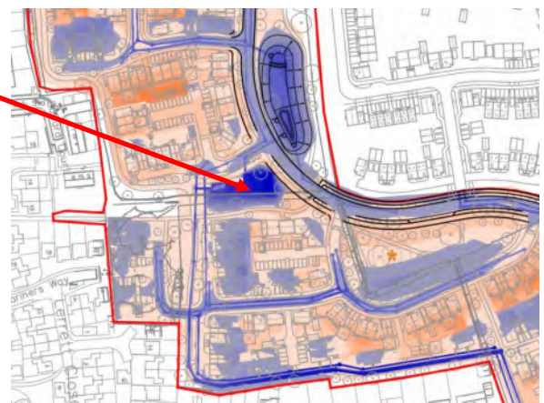
Phase A Cut & Fill Analysis P932/106 Aug '23
