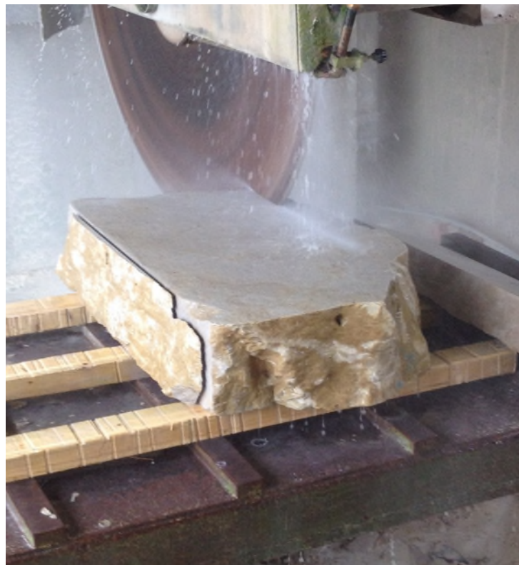
3. Block being 'squared up' on the saw at California.
