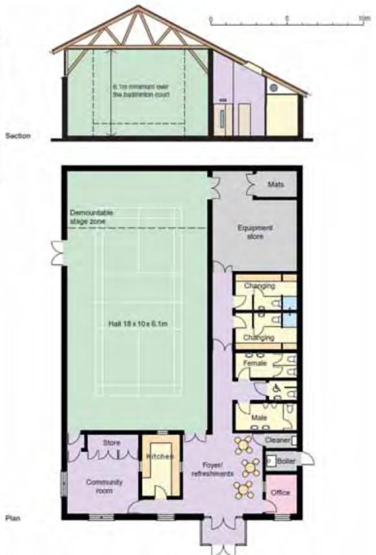
Plan and section of an economically designed hall layout. The double set of corridor doors would allow the changing rooms to be used for stage productions.
